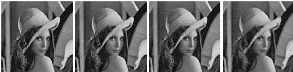
Fig. 11. Lena image blurred with out-of-focus kernel of radius 3, and then corrupted by Gaussian noise with \sigma = 5 and random-valued impulse noise with r = 10\%, 25\%, 40\% , and 55\% respectively. From left to right : The restored image by our method with PSNRs 27.2dB, 27.0dB, 26.7dB, and 25.6dB respectively. The parameters we used are [\alpha = 0.05, \beta = 0.05, \epsilon = 0.0002] , [\alpha = 0.01, \beta = 0.005, \epsilon = 0.0002] , [\alpha = 0.01, \beta = 0.005, \epsilon = 0.0002] , [\alpha = 0.01, \beta = 0.01, \epsilon = 0.0001] respectively. The functional minimized is (13) for p = 2 for s = 10\% and (13) for p = 1 for others according to Table II. The \tilde{\sigma} is 6.5, 7.0, 8.4 and 11.9 respectively.
