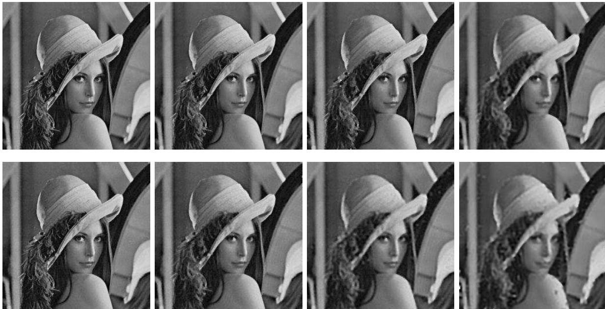
Fig. 8. Lena image blurred with out-of-focus kernel of radius 3, and then corrupted by random-valued noise with noise levels are 10%, 25%, 40%, and 55% respectively. Top : The restored image by our method, and the parameters we used are [\alpha = 0.0005, \beta = 0.0005, \epsilon = 0.001] , [\alpha = 0.001, \beta = 0.001, \epsilon = 0.0005] , [\alpha = 0.002, \beta = 0.002, \epsilon = 0.0005] , [\alpha = 0.005, \beta = 0.005, \epsilon = 0.0001] respectively. Bottom : The restored image by the full variational method, and the parameters we used are [\alpha = 0.001, \beta = 0.001, \epsilon = 0.0005] , [\alpha = 0.005, \beta = 0.005, \epsilon = 0.0005] , [\alpha = 0.005, \beta = 0.005, \epsilon = 0.00005] , [\alpha = 0.01, \beta = 0.01, \epsilon = 0.0001] respectively.
