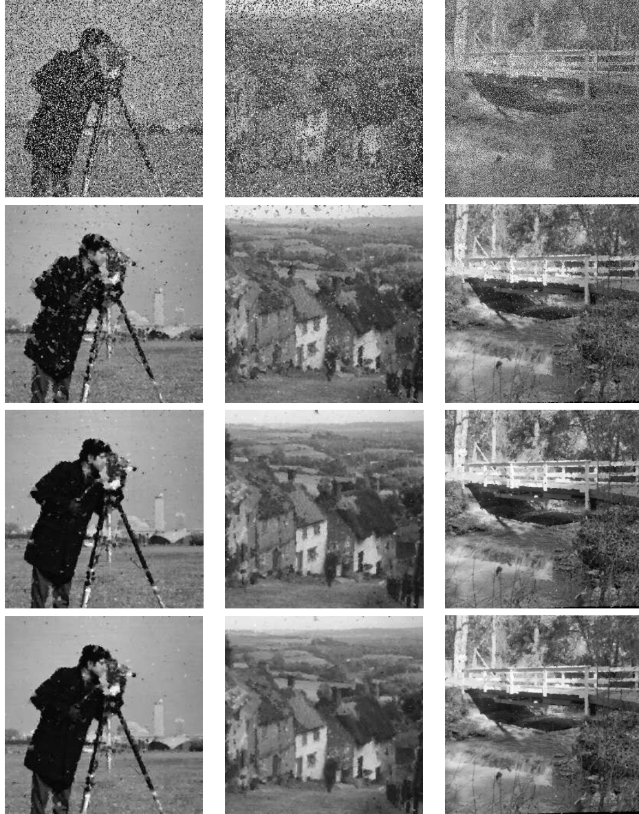
Figure 5: From top to bottom: images corrupted with 50% random-valued impulse noise, restored by ACWMF, restored by 2-phase variational method [8], and restored by Algorithm 3.
