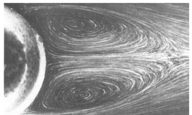
Fig. 8 Comparison of streamlines between the experiment and computation. Reprinted in part with permission from [42]. © (1956) The Physical Society of Japan.
