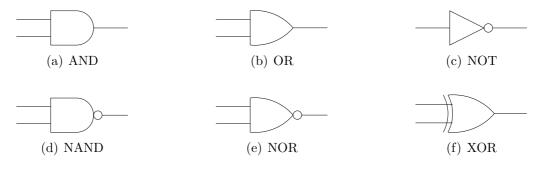
Figure 1: Six symbols of elementary logic gates
