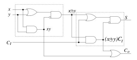
Figure 3: Full-adder:  $S = x \oplus y \oplus C_I, C_o = xy \lor (x \oplus y)C_I$
