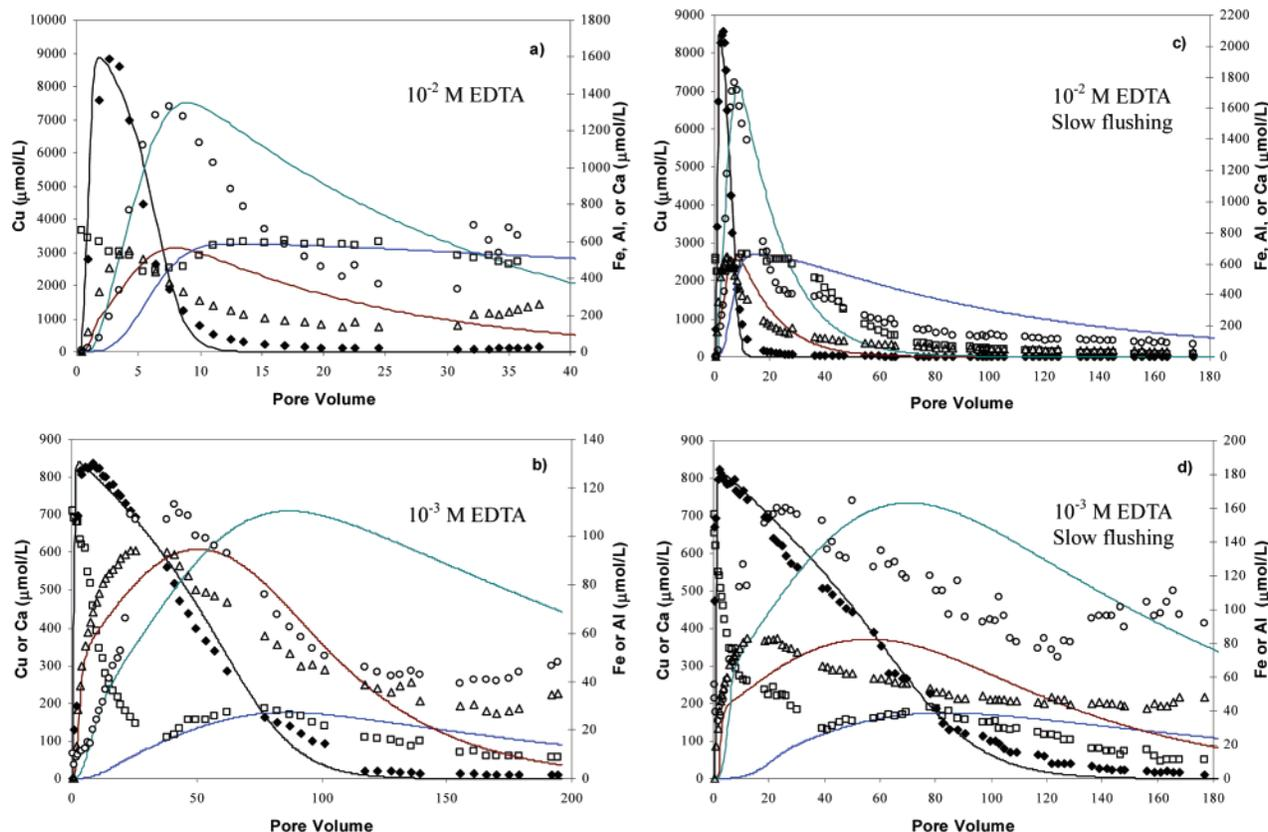
FIGURE 2. Breakthrough curves of Cu, Fe, Al, and Ca during EDTA-flushing of soils with aged Cu contamination: (a)  $10^{-2}$  M EDTA; (b)  $10^{-3}$  M EDTA; (c) slow flushing of  $10^{-2}$  M EDTA; (d) slow flushing of  $10^{-3}$  M EDTA (◆ Cu; △ Fe; ○ Al; □ Ca; lines are respective model simulations).
