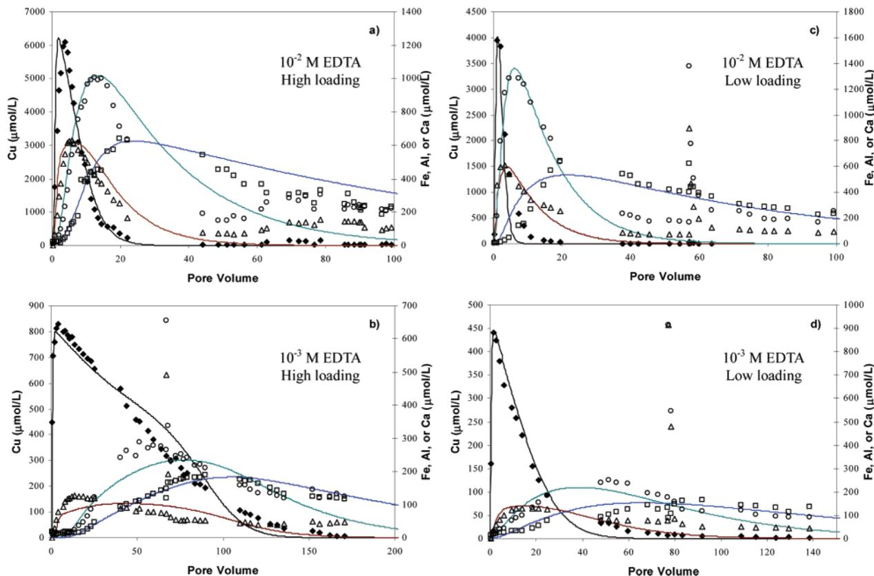
**FIGURE 1.** Breakthrough curves of Cu, Fe, Al, and Ca during EDTA-flushing of soils: (a)  $10^{-2}$  M EDTA, high Cu loading; (b)  $10^{-3}$  M EDTA, high Cu loading; (c)  $10^{-2}$  M EDTA, low Cu loading; (d)  $10^{-3}$  M EDTA, low Cu loading (◆ Cu; △ Fe; ○ Al; □ Ca; lines represent respective model simulations; obvious increase of concentrations in b–d upon 16-h flow interruption).
