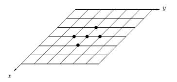
Figure 1.2: Two-dimensional grid on the unit square. The solid dots indicate the unknowns that are related at a typical grid point by the discrete equations (1.5).
