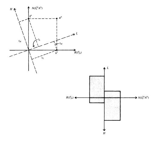
Figure 5.8: The top diagram shows the space  $\Omega^h$  decomposed along the (lowfrequency, high-frequency) axes and along the  $(\mathcal{R}(I_{2h}^h), N(I_{h}^{2h}A^h))$  axes. The initial error,  $\mathbf{e}^h$ , appears as a point with projections on all four axes. The lower diagram gives a schematic "energy budget" of the initial error. The error energy is divided between  $\mathcal{R}(I_{2h}^h)$  and  $N(I_{h}^{2h}A^h)$  and further divided between low- and high-frequency modes.
