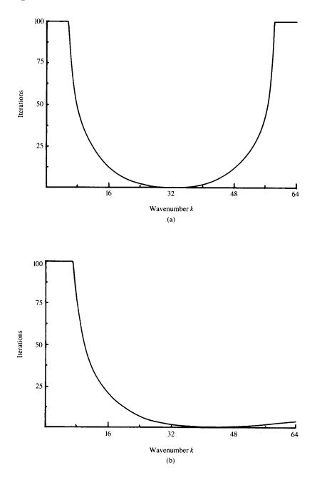
Figure 2.8: Weighted Jacobi method with (a)  $\omega = 1$  and (b)  $\omega = \frac{2}{3}$  applied to the one-dimensional model problem with n = 64 points. The initial guesses consist of the modes  $\mathbf{w}_k$  for  $1 \le k \le 63$ . The graphs show the number of iterations required to reduce the norm of the initial error by a factor of 100 for each  $\mathbf{w}_k$ . Note that for  $\omega = \frac{2}{3}$ , the damping is strongest for the oscillatory modes ( $32 \le k \le 63$ ).
