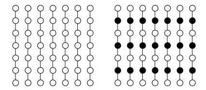
Figure 8.7: Semi-coarsening produced for a stretched mesh (or anisotropic) problem. Shown on the left is the grid with only the strong dependencies indicated. On the right, the final coarsening is displayed.
