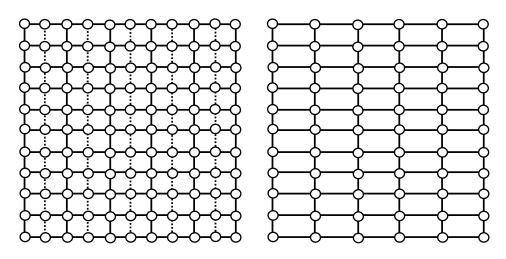
Figure 7.3: The original fine grid (left, solid and dashed lines) is semicoarsened in the x-direction by deleting the dashed lines (right).
