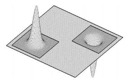
Figure 9.5: Two-spike solution of the composite grid problem based on a  $63 \times 63$  interior global grid, with mesh size  $h = \frac{1}{64}$ , and  $51 \times 51$  patches of mesh size  $\frac{h}{2} = \frac{1}{128}$  centered at  $(\frac{1}{4}, \frac{1}{4})$  and  $(\frac{3}{4}, \frac{3}{4})$ .
