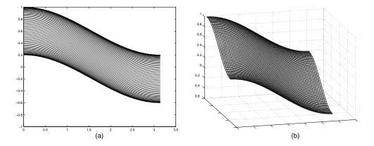
Figure 4.4: (a) Amplification factor,  $G(\theta_1, \theta_2)$ , for the weighted Jacobi method applied to the model problem in two dimensions, shown as individual curves of fixed  $\theta_1$  ( $\theta_1 = 0$  at the top and  $\theta_1 = \pi$  at the bottom). (b) Same amplification factor shown as a surface over the region  $[0, \pi] \times [0, \pi]$ . The picture is symmetric about both the  $\theta_1$ - and  $\theta_2$ -axes.
