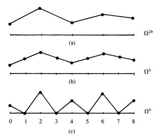
Figure 5.1: The action of  $A^h$  on the range of interpolation  $\mathcal{R}(I_{2h}^h)$ : (a) an arbitrary vector  $\mathbf{u}^{2h} \in \Omega^{2h}$ ; (b) the linear interpolant  $I_{2h}^h \mathbf{u}^{2h}$ ; and (c)  $A^h I_{2h}^h \mathbf{u}^{2h}$ , which is zero at the odd grid points on  $\Omega^h$ .
