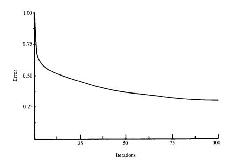
Figure 2.5: Weighted Jacobi method with  $\omega = \frac{2}{3}$  applied to the one-dimensional model problem with n = 64 points and an initial guess  $(\mathbf{v}_1 + \mathbf{v}_6 + \mathbf{v}_{32})/3$ . The maximum norm of the error,  $\|\mathbf{e}\|_{\infty}$ , is plotted against the iteration number for 100 iterations.
