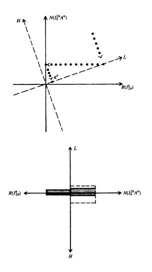
Figure 5.11: The top diagram shows the effect of several more fine-grid relaxations on the error. Once again, all high-frequency components are removed as indicated by a projection onto the L-axis. The lower diagram shows the corresponding changes in the energy budget.
