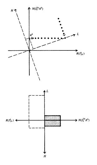
Figure 5.10: The top diagram shows the error after doing the remainder of the two-grid correction. All components in  $\mathcal{R}(I_{2h}^h)$  are eliminated as indicated by the projection onto the N-axis. The lower diagram shows the corresponding changes in the energy budget.
