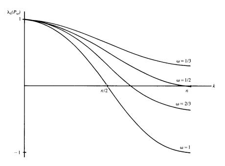
Figure 2.7: Eigenvalues of the iteration matrix  $R_{\omega}$  for  $\omega = \frac{1}{3}, \frac{1}{2}, \frac{2}{3}, 1$ . The eigenvalues  $\lambda_k = 1 - 2\omega \sin^2\left(\frac{k\pi}{2n}\right)$  are plotted as if k were a continuous variable on the interval  $0 \le k \le n$ . In fact,  $1 \le k \le n - 1$  takes only integer values.
