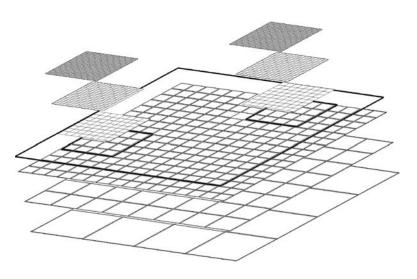
Figure 9.7: Side view of a global  $15 \times 15$  grid with two coarser supporting grids and three successively finer local grids.
