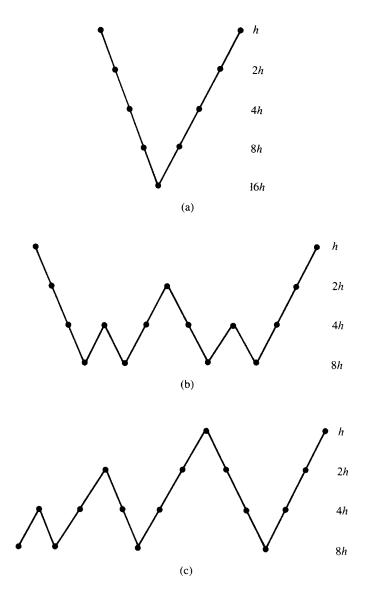
Figure 3.6: Schedule of grids for (a) V-cycle, (b) W-cycle, and (c) FMG scheme, all on four levels.
