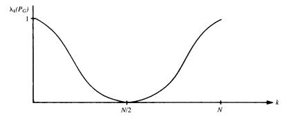
Figure 2.10: Eigenvalues of the Gauss–Seidel iteration matrix. The eigenvalues  $\lambda_k = \cos^2\left(\frac{k\pi}{n}\right)$  are plotted as if k were a continuous variable on the interval  $0 \le k \le n$ .
