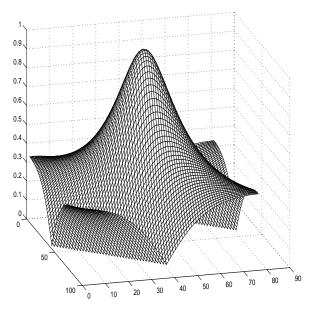
Figure 4.5: Amplification factor,  $|G(\theta_1, \theta_2)|$ , for the Gauss–Seidel method applied to the model problem in two dimensions, shown as a surface over the region  $[-\pi, \mathbf{a}, \pi] \times [\pi, \pi]$ .
