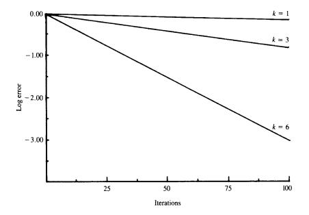
Figure 2.4: Weighted Jacobi iteration with  $\omega = \frac{2}{3}$  applied to the one-dimensional model problem with n = 64 points and with initial guesses  $\mathbf{v}_1$ ,  $\mathbf{v}_3$ , and  $\mathbf{v}_6$ . The log of  $\|\mathbf{e}\|_{\infty}$  is plotted against the iteration number for 100 iterations.
