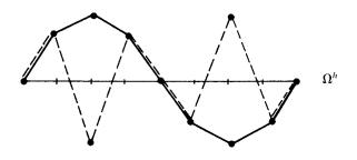
Figure 5.3: A pair of complementary modes on a grid with n = 8 points. The solid line shows the k = 2 mode. The dashed line shows the k' = n - k = 6 mode.
