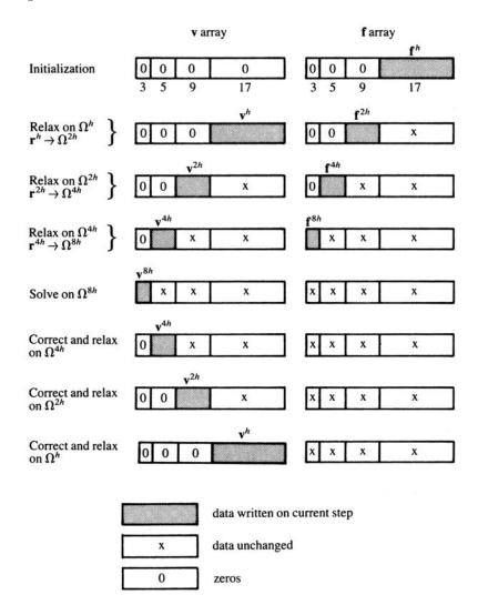
Figure 4.1: Illustration of the course of a four-level (n = 16) V-cycle showing changes in the data arrays. The **v** and **f** arrays hold the solution vectors and right-side vectors, respectively, in the four grids.
