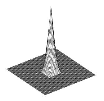
Figure 10.3: A typical basis function  $\epsilon_{i,j}^h(x,y)$  for the space  $H^h$ . It is nonzero, only on the patch of four elements that have  $(x_i, y_j)$  as a node.
