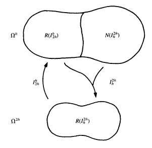
Figure 5.7: Schematic drawing of the space of fine-grid vectors,  $\Omega^h$ ; the space of coarse-grid vectors,  $\Omega^{2h}$ ; and their subspaces and the intergrid transfer operators,  $I_{2h}^h$  and  $I_h^{2h}$ .
