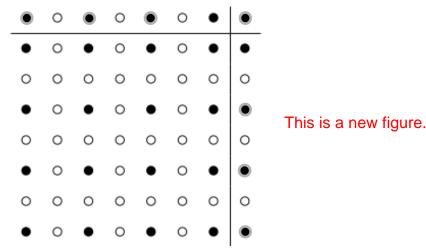
Figure 8.6: Second coloring pass for the nine-point Laplacian problem with periodic boundary conditions. The added C-points are shown in the final coloring as black dots with thick gray outlines.
