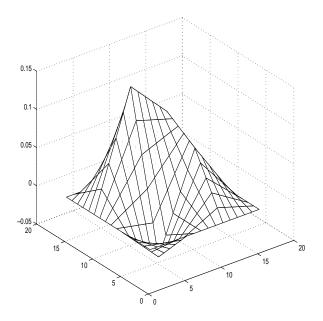
Figure 10.2: A typical function in the space  $H^h$  used to approximate the solution to the problem. It is zero on  $\partial\Omega$ , continuous on  $\Omega$ , and bilinear within each of the nine elements pictured.
