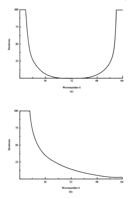
Figure 2.11: Gauss-Seidel iteration matrix applied to the model problem with n = 64 points. The initial guesses consist of (a) the eigenvectors of the iteration matrix  $R_G$  with wavenumbers  $1 \le k \le 63$  and (b) the eigenvectors of A with wavenumbers  $1 \le k \le 63$ . The figure shows the number of iterations required to reduce the norm of the initial error by a factor of 100 for each initial guess.
