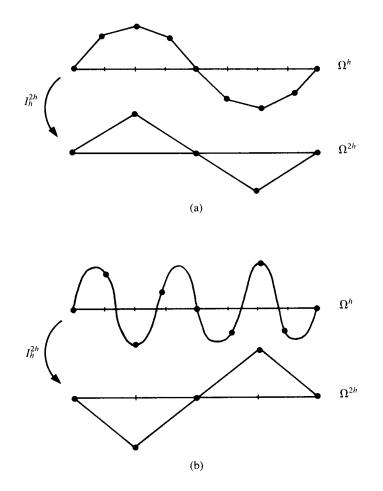
Figure 5.2: The full weighting operator  $I_h^{2h}$  acting on (a) a smooth mode of  $\Omega^h$  (k = 2 and n = 8) and (b) an oscillatory mode of  $\Omega^h$  (k = 6 and n = 8). In the first case, the result is a multiple of the k = 2 mode on  $\Omega^{2h}$ . In the second case, the result is a multiple of the n - k = 2 mode on  $\Omega^{2h}$ .
