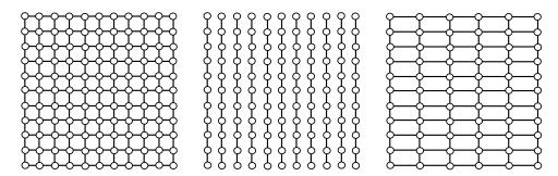
Figure 7.5: It is possible to combine line relaxation and semicoarsening. The original grid (left) is viewed as a collection of pencils for line relaxation in the y-direction (center) and semi-coarsened in the x-direction (right).
