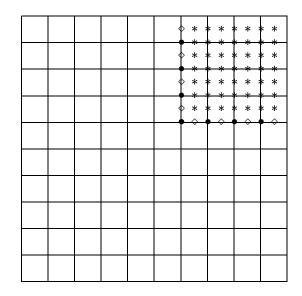
Figure 9.4: Composite grid on a two-dimensional domain. The coarse-grid points are at the intersection of the solid horizontal and vertical lines. The local fine grid consists of \* points. Interface points coinciding with coarse-grid points are marked by  $\bullet$ . The new slave points ( $\diamond$ ) are interface points that do not overlay a fine-grid point. Boundary points have been omitted.
