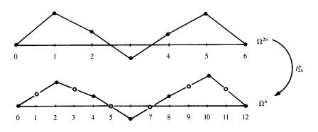
Figure 3.2: Interpolation of a vector on coarse grid  $\Omega^{2h}$  to fine grid  $\Omega^{h}$ .
