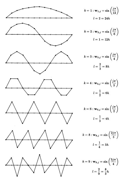
Figure 2.6: Graphs of the Fourier modes of A on a grid with n = 12 points. Modes with wavenumbers k = 1, 2, 3, 4, 6, 8, 9 are shown. The wavelength of the kth mode is  $\ell = \frac{24h}{k}$ .
