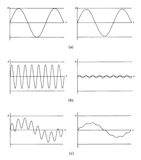
Figure 2.9: Weighted Jacobi method with  $\omega = \frac{2}{3}$  applied to the one-dimensional model problem with n = 64 points and with an initial guess consisting of (a)  $\mathbf{w}_3$ , (b)  $\mathbf{w}_{16}$ , and (c)  $(\mathbf{w}_2 + \mathbf{w}_{16})/2$ . The figures show the approximation after one iteration (left side) and after 10 iterations (right side).
