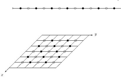
Figure 2.1: A one-dimensional grid (top) and a two-dimensional grid (bottom), showing the red points ( $\circ$ ) and the black points ( $\bullet$ ) for red-black relaxation.
