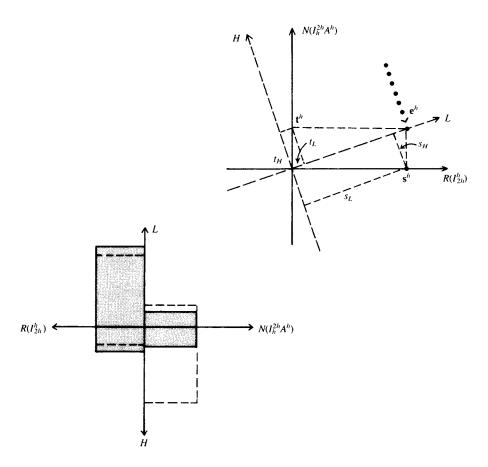
Figure 5.9: The top diagram shows the effect of several fine-grid relaxation sweeps. Assuming that all oscillatory components are eliminated, the error is projected onto the low-frequency axis (L). The lower diagram shows the corresponding changes in the energy budget. Dashed lines indicate the previous energy budget. Shaded areas show the current budget.
