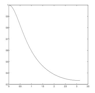
Figure 4.2: The amplification factor,  $|G(\theta)|$ , for the Gauss–Seidel method applied to the one-dimensional problem -u''(x) = f(x). The graph is symmetric about  $\theta = 0$ . The smoothing factor is  $\mu = |G(\frac{\pi}{2})| = \frac{1}{\sqrt{5}} = 0.45$ .
