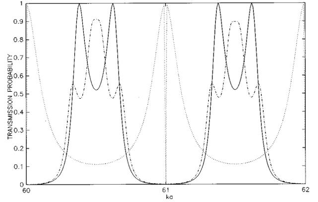
FIG. 3. Transmission probability as a function of the energy of incident electrons ( $E_F=\hbar^2k^2/2m$ ) for  $\epsilon=0.25$ ,  $a=1 \mu\text{m}$ ,  $\alpha=1.8$ ,  $\chi_2=\pi/6$ , and  $\phi=0$ . The dotted line corresponds to the absence of the SO interaction and Zeeman coupling, the solid line corresponds to the presence of the SO interaction only, and the dash-dotted line corresponds to the presence of both the SO interaction and the Zeeman coupling of  $B=30 \text{ G}$ .
