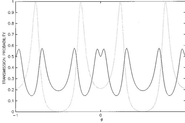
FIG. 2. Transmission probability as a function of the AB flux for  $\epsilon=0.25$ ,  $ka=60.239$ ,  $a=1 \mu\text{m}$ , and  $\chi_2=\pi/6$ . The dotted and the solid lines are associated with the absence of and the presence of the SO interaction of  $\alpha=1.8$ , respectively.
