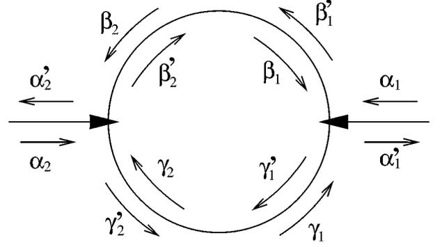
FIG. 1. Schematic representation of the electronic waves propagating through the ring connected to current leads. The right junction is located at  $\theta=0$  and the left junction at  $\theta=\pi$ , with the upper branch lying within  $(0, \pi)$  and the lower branch within  $(\pi, 2\pi)$ .
