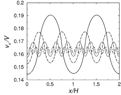
FIG. 5. Slip profiles at differently patterned solid surfaces. The pattern period  $P=w_A+w_B$  varies from  $H$  to  $H/8$ , with equal stripe widths ( $w_A=w_B$ ). The solid line is for  $P/H=1$ , the dashed line for  $P/H=1/2$ , the dotted line for  $P/H=1/4$ , and the dash-dotted line for  $P/H=1/8$ .
