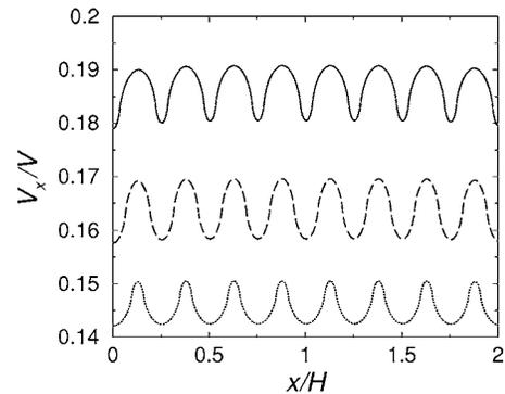
FIG. 6. Slip profiles at differently patterned solid surfaces. The pattern period  $P=w_A+w_B$  equals  $H/4$ , with  $w_A/w_B$  varying from  $1/3$  (solid line) to  $1$  (dashed line) and to  $3$  (dotted line).
