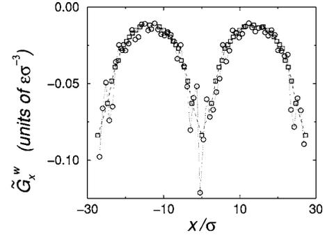
FIG. 1. Hydrodynamic tangential wall force  $\tilde{G}_x^w(x)$  at the lower fluid-solid interface. The circles denote  $\tilde{G}_x^w(x)$  directly measured in the MD simulation; the squares denote  $\tilde{G}_x^w(x)$  calculated from  $\beta(x)$  and the measured  $v_x^{slip}(x)$ .
